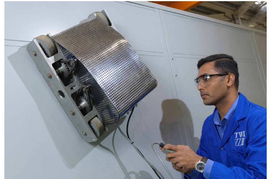
Mahesh Dissanayake working with a payload carrying magnetic adhesion climbing robot
