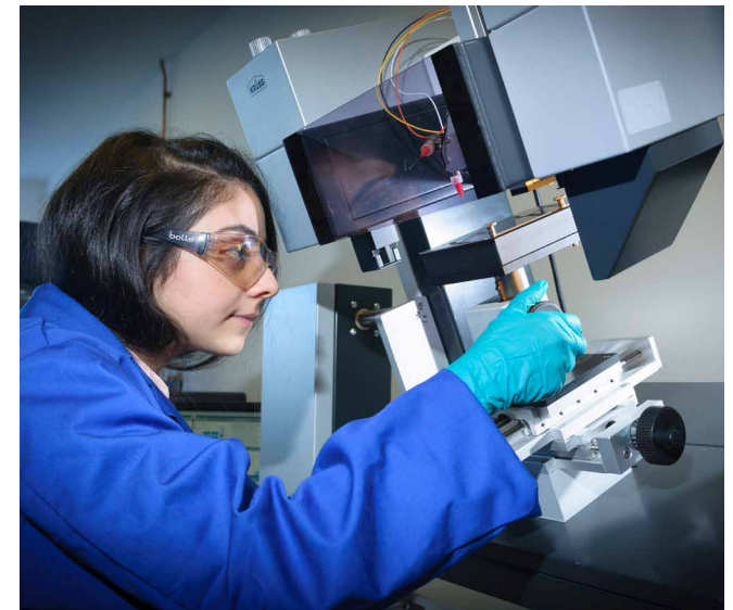
Taraneh Moghim characterises surface repellency of super-hydrophobic coatings
